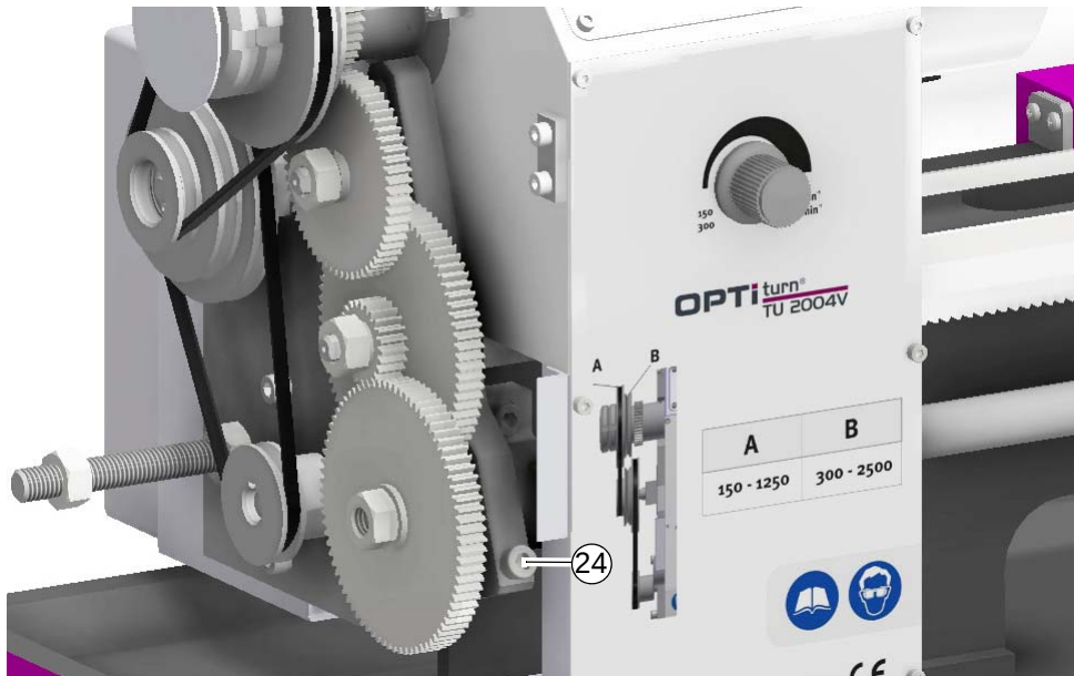
Img.4-8: Locking screw quadrant
