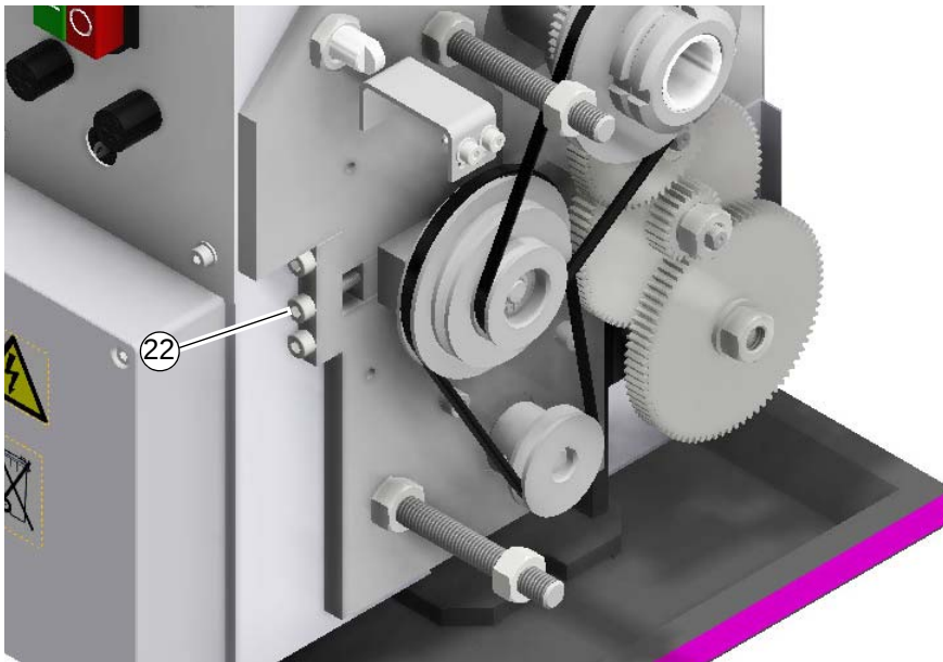
Img.4-6: Synchronous belt position change
